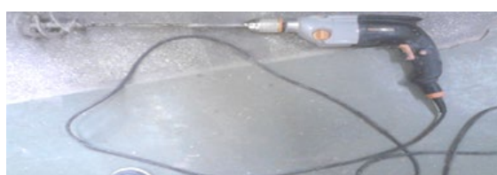
Fig. 28. The equipment used to homogenize the mixture
