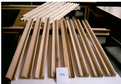
Fig. 43. Test pieces milled from beech wood
