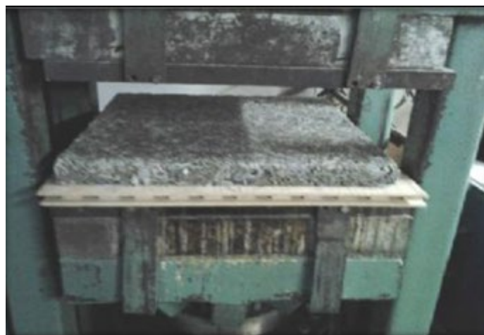
Fig. 33. Pressing of composites (Brenci et al. 2014)
