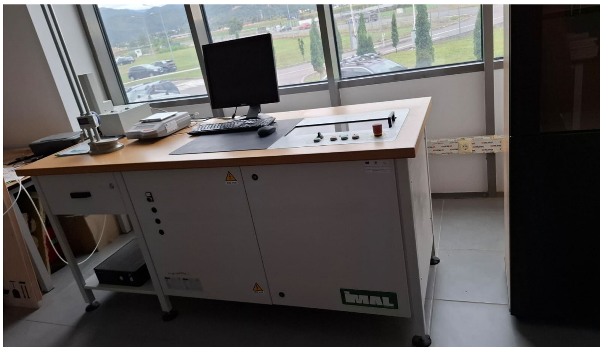
Fig. 10. DPX300 equipment for measuring the vertical density profile
