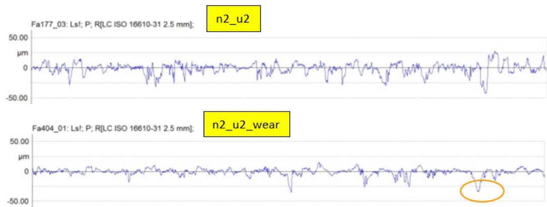
Fig. 58. Roughness profiles of each group combination, rotation speed-feed speed comparing the effect of tool condition (sharpened and after wear). Raised fibers are marked with red, deep isolated val-leys are marked with yellow ellipse (Brenci and Gurău 2024)
