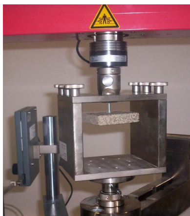
Fig. 7. Mechanical test for testing the screw holding strength
