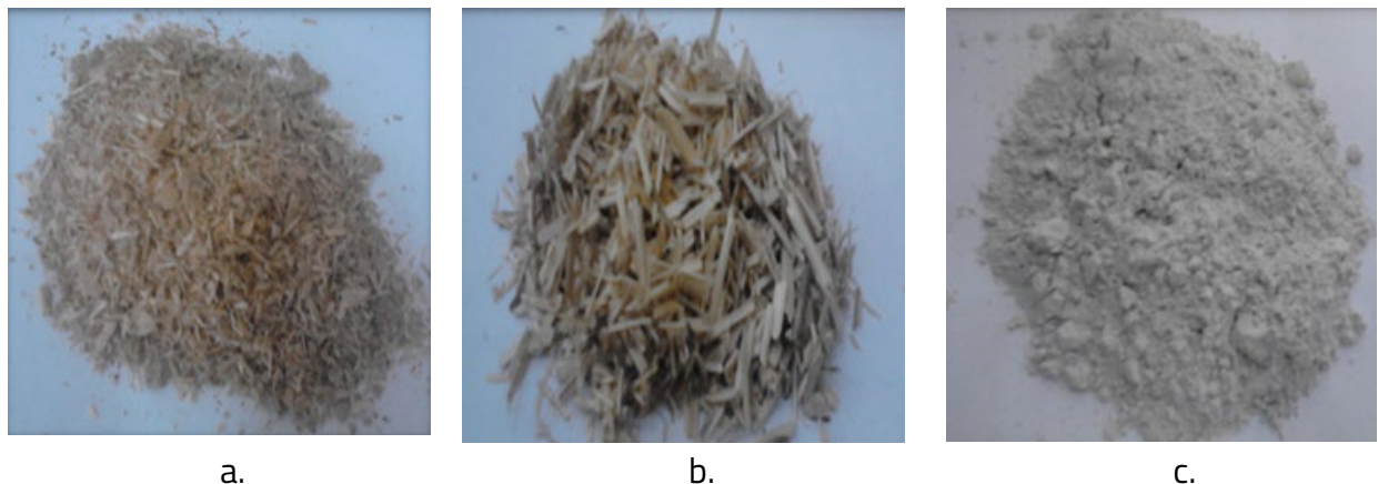
Fig. 32. Materials used in the manufacturing of composites (Brenci et al. 2014) (a) wood shavings; (b) hemp particles; (c) gypsum
