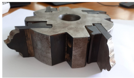
Figure 2. The profile cutterhead used in the milling process.
