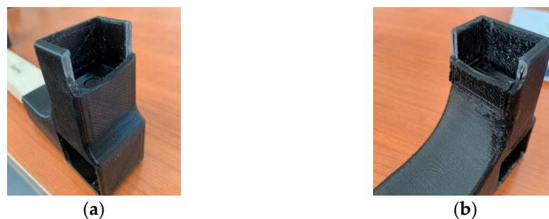
Figure 14. Connector failure: (a) Under tensile load; (b) Under compression load.
