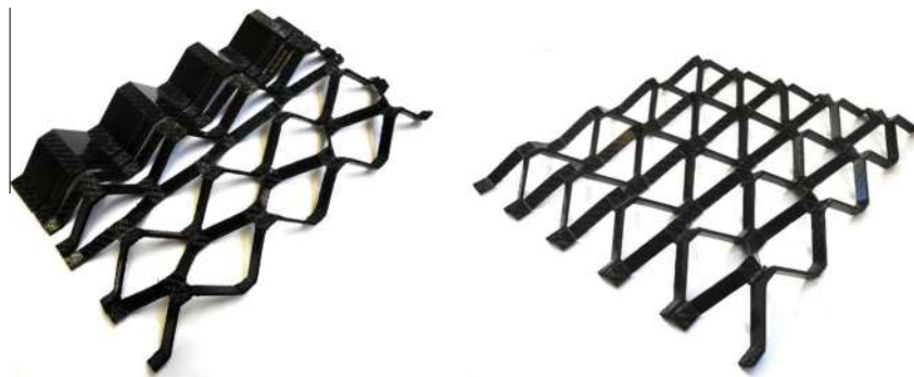
Fig. 3. CPET material in the process of expansion from a corrugation to a lattice truss structure (left) and final result of an expanded lattice truss core structure made of CPET with \beta = \omega = 45^\circ , l_1 = 28.28 mm, l_2 = 10 mm, t = 1.8 mm, d = 9.7 mm and c = 2 mm (right).
