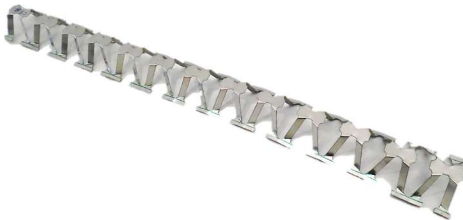
Figure 3. A strip of mechanically expanded perforated corrugated structure—pyramidal cellular structure.
