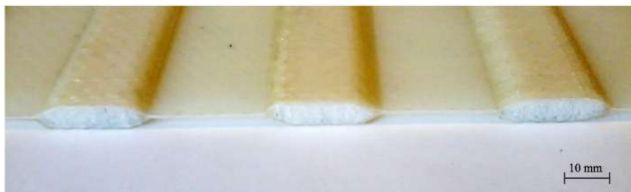
Fig. 4. Cross-section within the resulted consolidated plate with alternative monolithic and sandwich sections.
