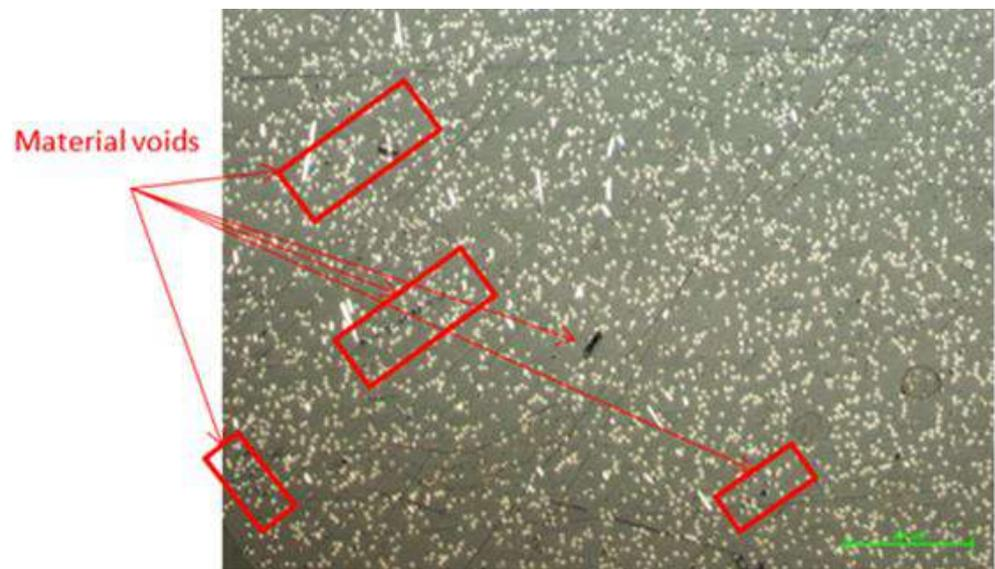
**Figure 11.** Ultrafuse PET CF15—Transversal view of the filament—Scale 100× (Scale length 200 μm)
