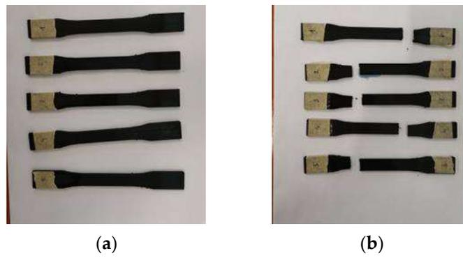
Figure A6. Longitudinal Tensile Specimens C\_15\_25: (a) Before testing; (b) After testing.
