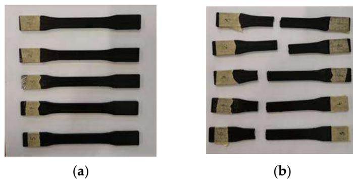
Figure A8. Longitudinal Tensile Specimens C\_25\_25: (a) Before testing; (b) After testing.
