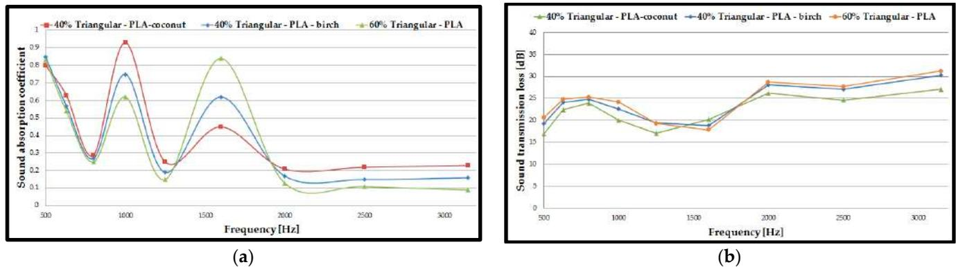
**Figure 10.** Acoustic test results of 3D-printed single panels with holes: (a) Sound absorption coefficient of 40% triangular-PLA-coconut; 40% triangular-PLA-birch and 60% triangular-PLA; (b) Sound transmission loss of 40% triangular-PLA-coconut; 40% triangular-PLA-birch and 60% triangular-PLA.
