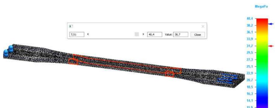
**FIGURE 11** Specimen zone where stress value is equal with ultimate tensile strength (P50\_45 specimen) [Color figure can be viewed at [wileyonlinelibrary.com](http://wileyonlinelibrary.com)]
