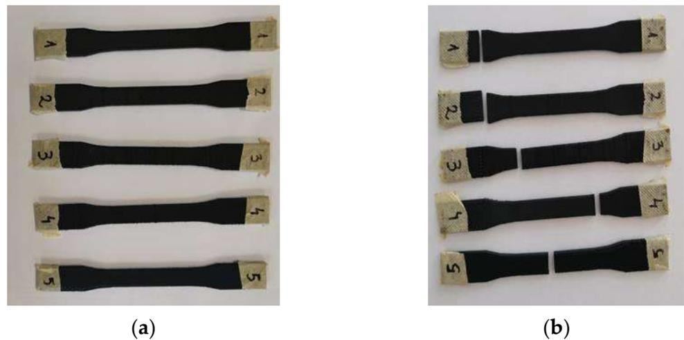
**Figure 8.** Thickness Direction Tensile Specimens C\_15\_100: (a) Before testing; (b) After testing.
