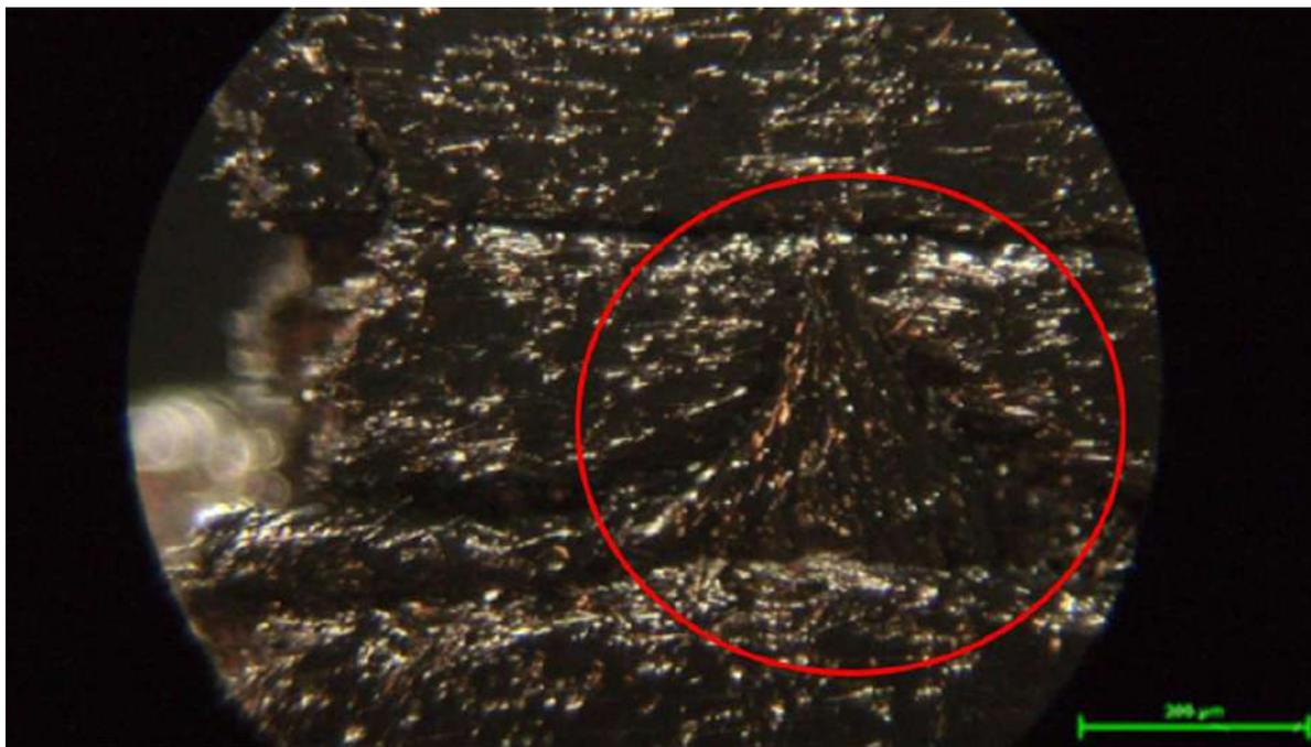
**Figure 23.** Specimens–Manufacturing defects–Inadequate material deposition (Scale 100×)–Scale length 200 μm–Nikon T1-SM.
