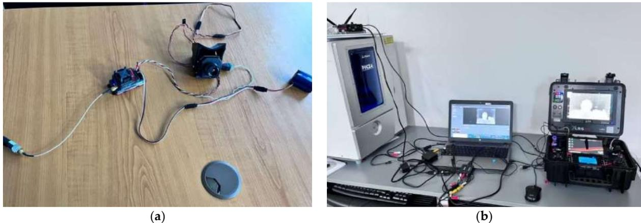
**Figure 17.** Testing the thermal module: (a) connecting the thermal module—smart antenna—battery—ground control station receiver; (b) image transmitted by the thermal module.
