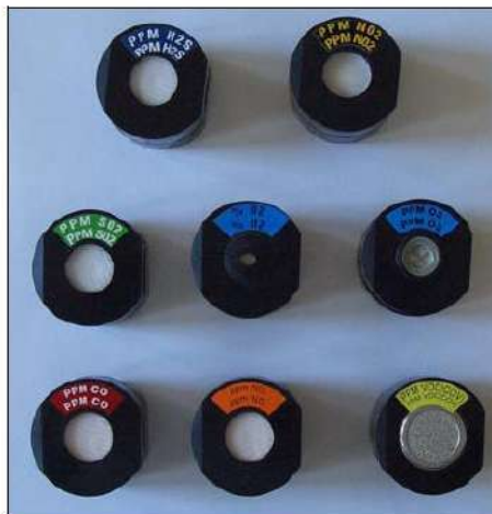
Fig. 7 The OLDHAM MX21 measurement cells
