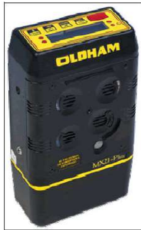
Fig. 6 The OLDHAM MX21 Plus portable multi-gas detector
