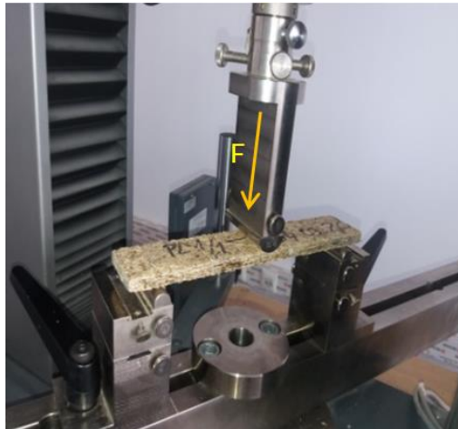
Fig. 5. Bending strength test
