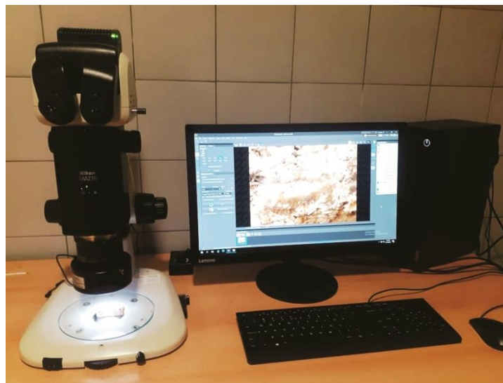
Fig. 8. NIKON SMZ 18-LOT2 stereo microscope, used for microscopic analysis of the panels' structure
