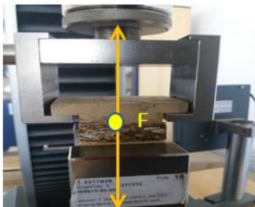
Fig. 6. Internal bond test
