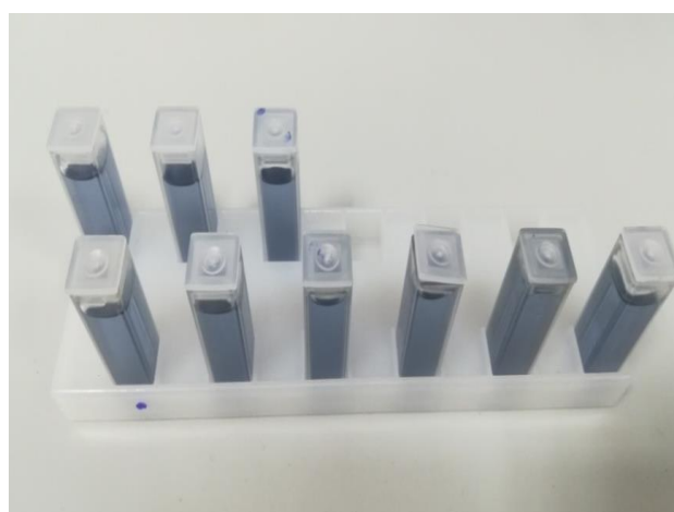
Figure 8.5 Preparation of Samples for Total Polyphenol Content Determination Using Folin-Ciocalteu Reagent
