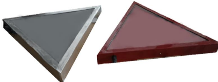
Fig.4.1. The two physical models of the red and black absorber plate collectors
