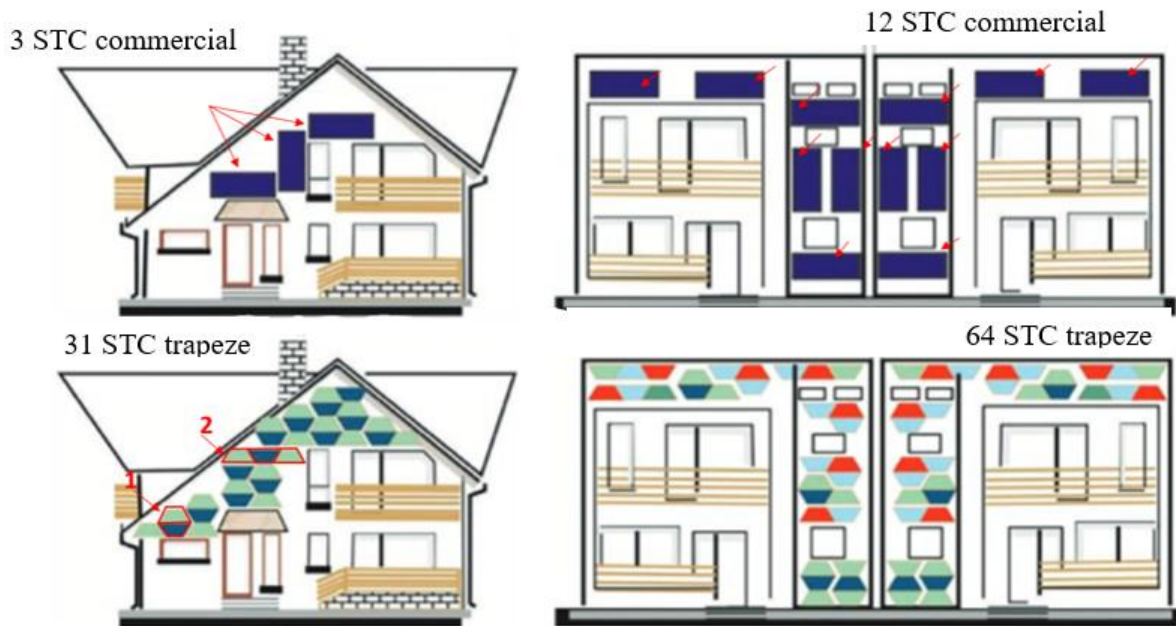
Fig. 1.6. Comparison of commercial vs. trapezoidal collector solar facades (Vişa et.al., 2017)
