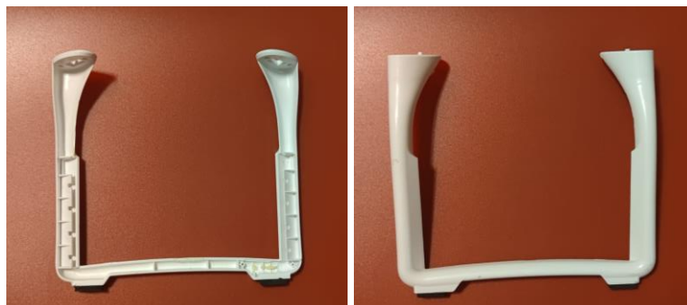
Figure 15 Landing Gear DJI Phantom 3 Pro– view from inside and outside (relative to mounting mode) [BLA24B]
