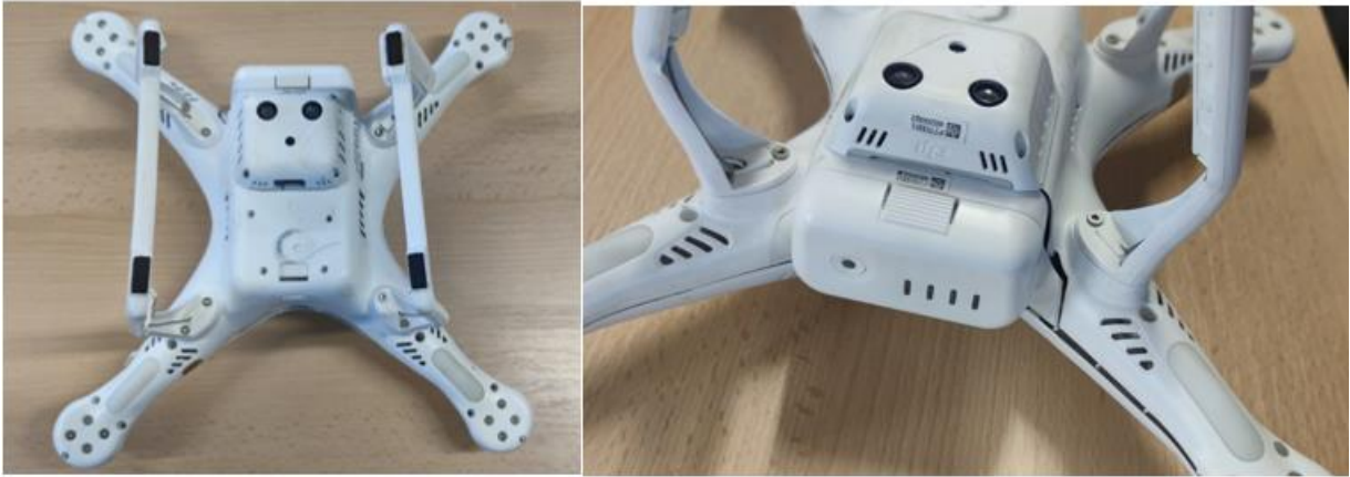
Figure 24 DJI Phantom 3 Pro – drone test with original parts – visual inspection of the structure after tests [BLA24B]
