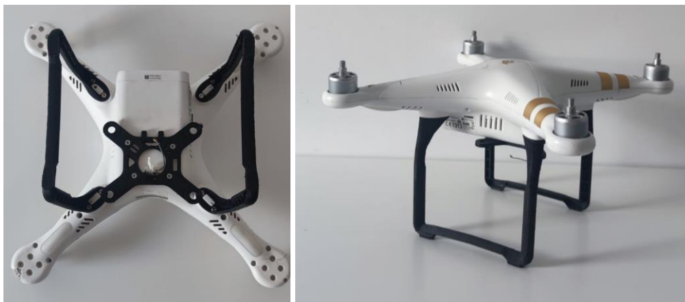
Figure 23 DJI Phantom 3 Pro – drone after the mounting of the redesigned and remanufactured parts [BLA24B]
