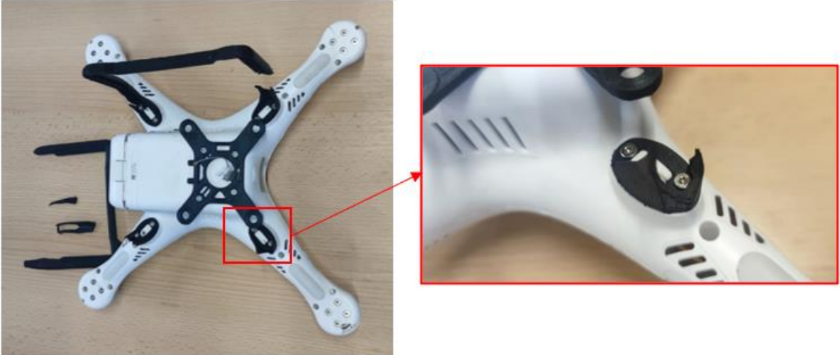
Figure 25 DJI Phantom 3 Pro – drone test with remanufactured parts – visual inspection of the structure after tests [BLA24B]
