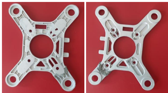
Figure 16 Gimbal Support Plate DJI Phantom 3 Pro– v view from inside and outside (relative to mounting mode) [BLA24B]
