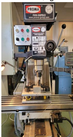
Figure 5.72 The dynamometer mounted on the table of milling machine-tool type PROMA FHV-50PD/2
