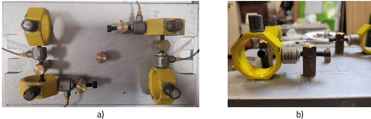
Figure 5.3. Force transducers mounting: a) in rings; b) detailed mounting
