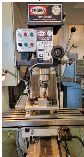
Figura 5.72 The dynamometer mounted on the Tabel of milling machine-tool type PROMA FHV-50PD/2
