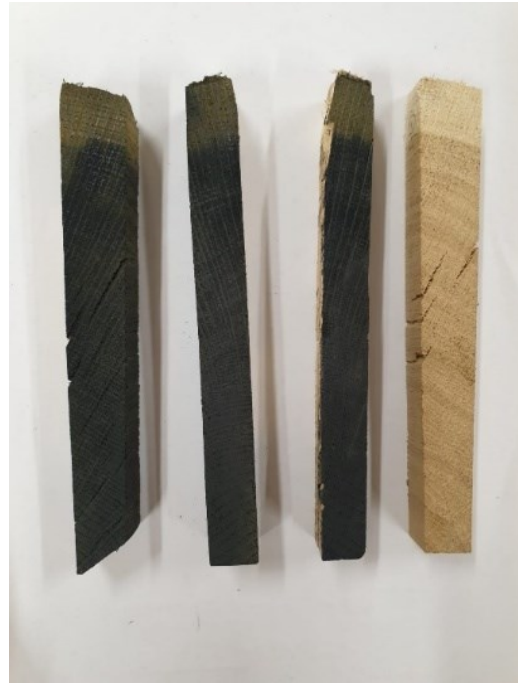
Fig. 4.15 Color change of Turkey oak wood (a) and Sessile oak wood (b) after application of FeCl_3
