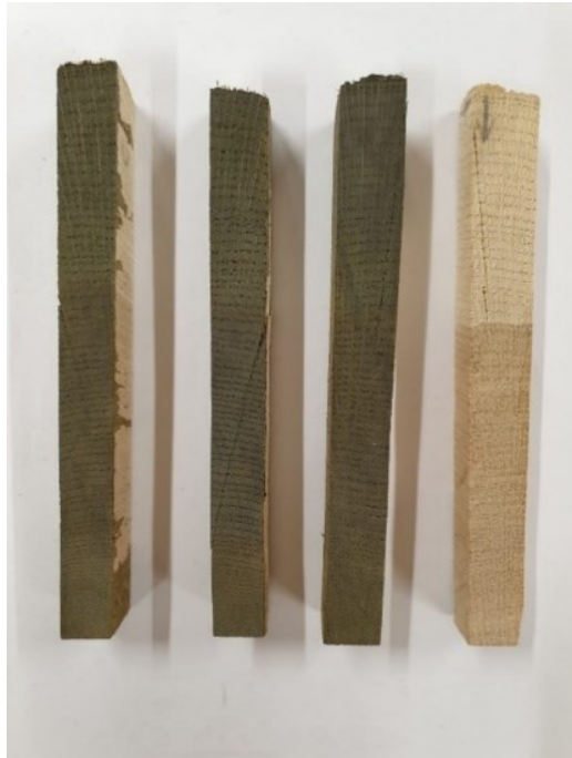
Fig. 4.15 Color change of Turkey oak wood (a) and Sessile oak wood (b) after application of FeCl_3
