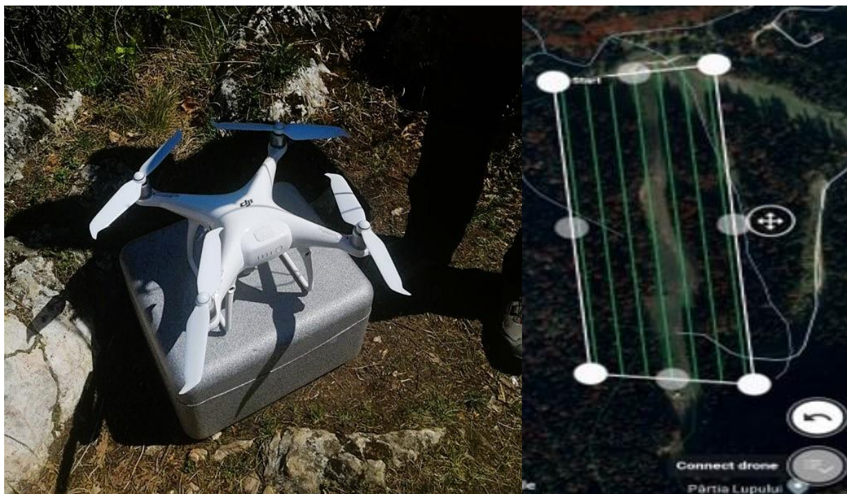
Fig. 3.2 - The drone used, the Phantom 4 Pro v2 model (photo on the left), and establishing the overflight route over the target trees (photo on the right) (Ciocîrlan 2022)
