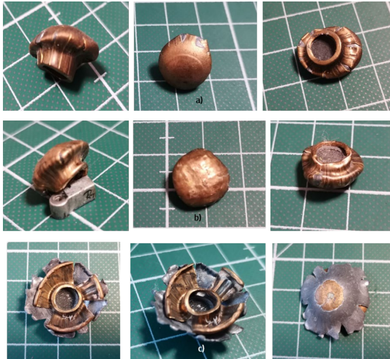
Figure 5.10 Projectile deformation after impact: a) PE-RCP-S configuration; b) PE-RCP-F configuration; c) PE-RCP-B configuration
