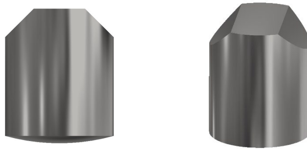
Figure 1.5 Fragment simulating projectile (FSP)
