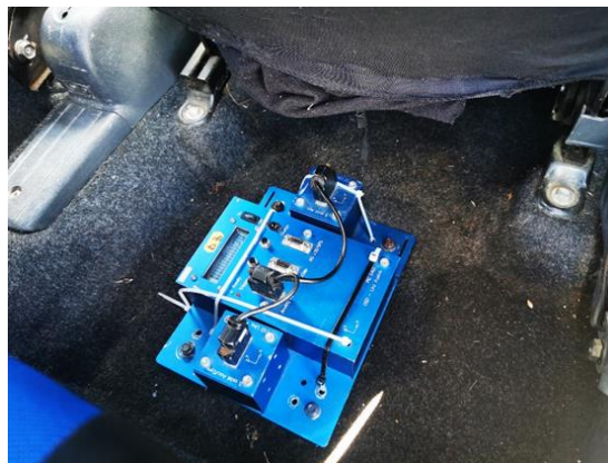
Figure 4.4 Installation location of the PicDAQ 4 system
