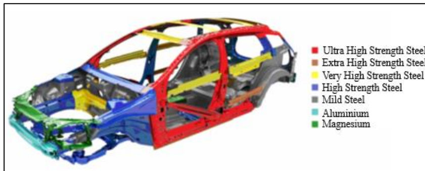
Figure 2.4 Materials from which a vehicle body is made [22]
