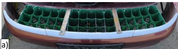
Figure 5.4 a) Plastic support of the shock absorption system ; b) Shock absorption system
