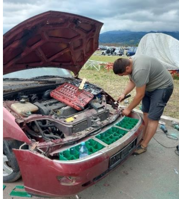
Figure 5.7 Installation of the energy-absorbing system
