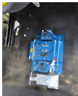
Figure 5.9 Area for installing the PicDAQ 4 accelerometer
