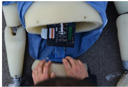
Figure 5.10 Installation of the PicDAQ 5 accelerometer inside the dummy's thorax
