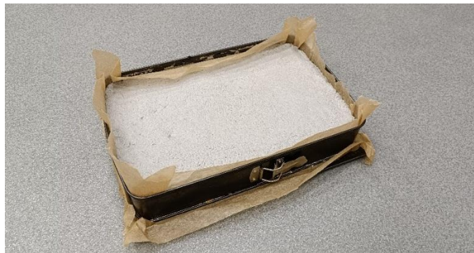
Figure 5. Raw material mixture (molding process) of the wet-process foam-type composite panels.
