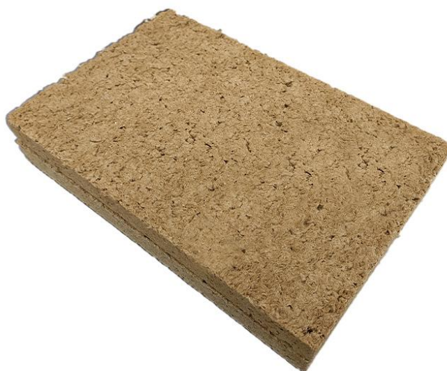
Figure 20. Foam-type composites made from recycled cardboard, sodium bicarbonate, baking powder, and vinegar as foaming agents.
