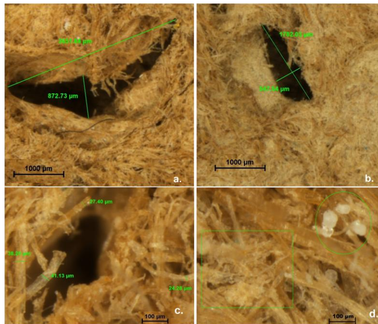
Figure 17. Measurements at 30 × magnification of the composites UcSCs 100-100 and UcSCs 100-200: a. 3.5 wt% corn starch; b. 7 wt% corn starch; c. Fiber size measurements at 180 × magnification; d. Fiber adhesion (squared area) and corn starch presence (circled area) at 300 × magnification.
