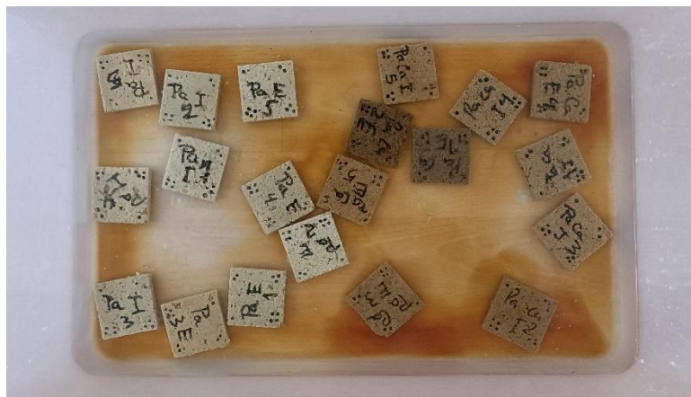
Figure 9. Water immersion of the specimens for the dimensional stability assessment.
