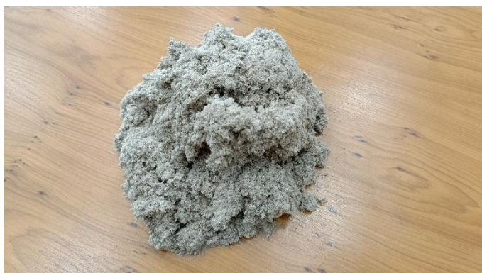
Figure 6. Raw material mixture of the dry-process foam-type composite panels.
