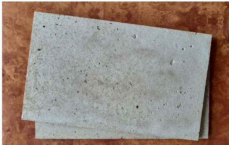
Figure 13. Final foam-type composite panel fabricated from recycled cardboard with foaming and binding agents: sodium bicarbonate and corn starch.
