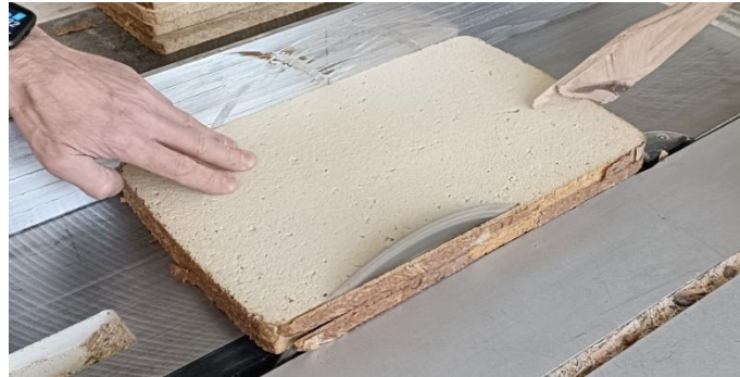
Figure 8. The final composite panel after cutting to size using a planner circular saw.
