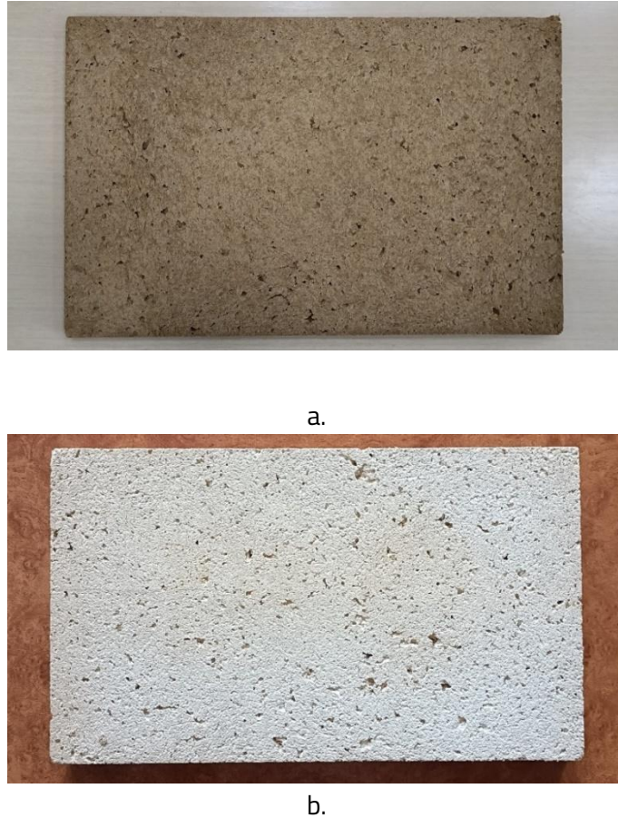
Figure 28. Foam-type composite panels made from recycled cardboard using sodium bicarbonate and yeast as foaming agents via wet and dry-process methods.
