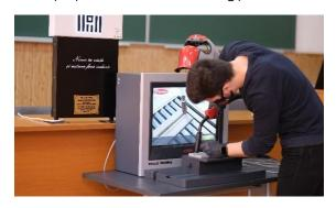
The *Virtual Welding* simulator is a system designed to train and improve the practical skills needed by the students in the specialization of Welding Engineering.
