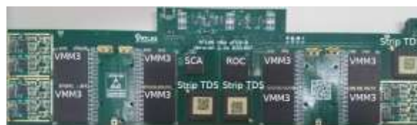
Photo of sFEB, Frontend and backend electronics for the New Small Wheel Upgrade of the ATLAS muon spectrometer, TWEPP 2018, edited
